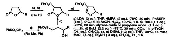
A procedure for the preparation of  $\alpha$ -substituted  $\beta$ -phenylsulfonyl dihydrofurans has been recently reported:
